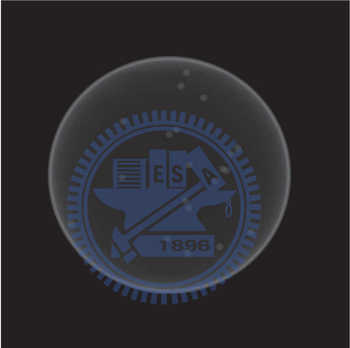
Figure 4.3: The simulated X-ray image of the phantom data. 180 emulated X-ray images were generated. The size of each image is 512 \times 512 pixels, the rotation angle between two consecutive images is 1^\circ , and the ranges of the vertical and horizontal errors are \pm 20 pixels.
