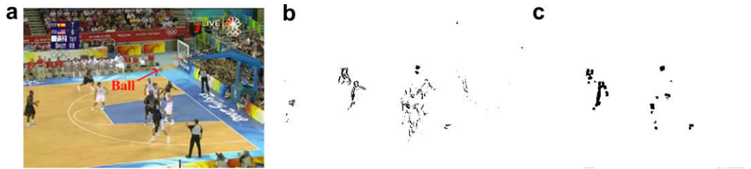
Fig. 11. Illustration of ball pixel detection. (a) Source frame; (b) moving pixels and (c) extracted ball pixels.
