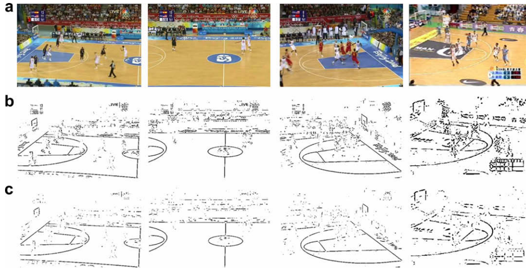
Fig. 8. Sample results of white line pixel detection. (a) Original frame; (b) without line-structure constraint and (c) with line-structure constraint.
