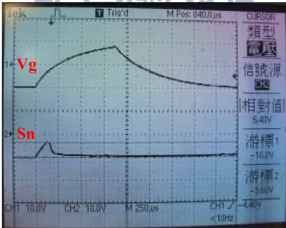
Fig. 3-17(b) \tau_{\text{delay}} is 300us
