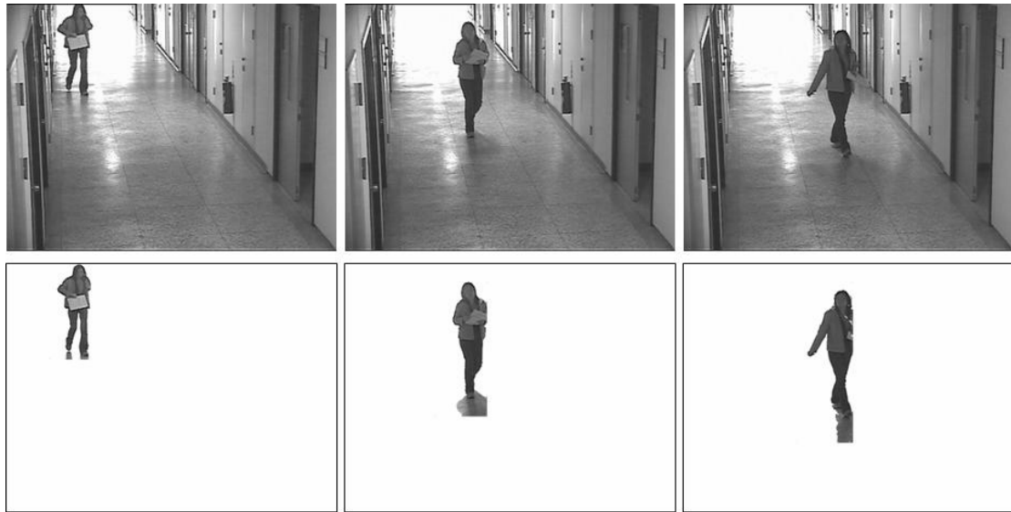
Fig. 2.1.1 (a1)(b1)(c1) Original images at (a) frame 11 (c) frame 17 (e) frame 20 (a2)(b2)(c2) Tracking results at (b) frame 11 (d) frame 17 (f) frame 20
