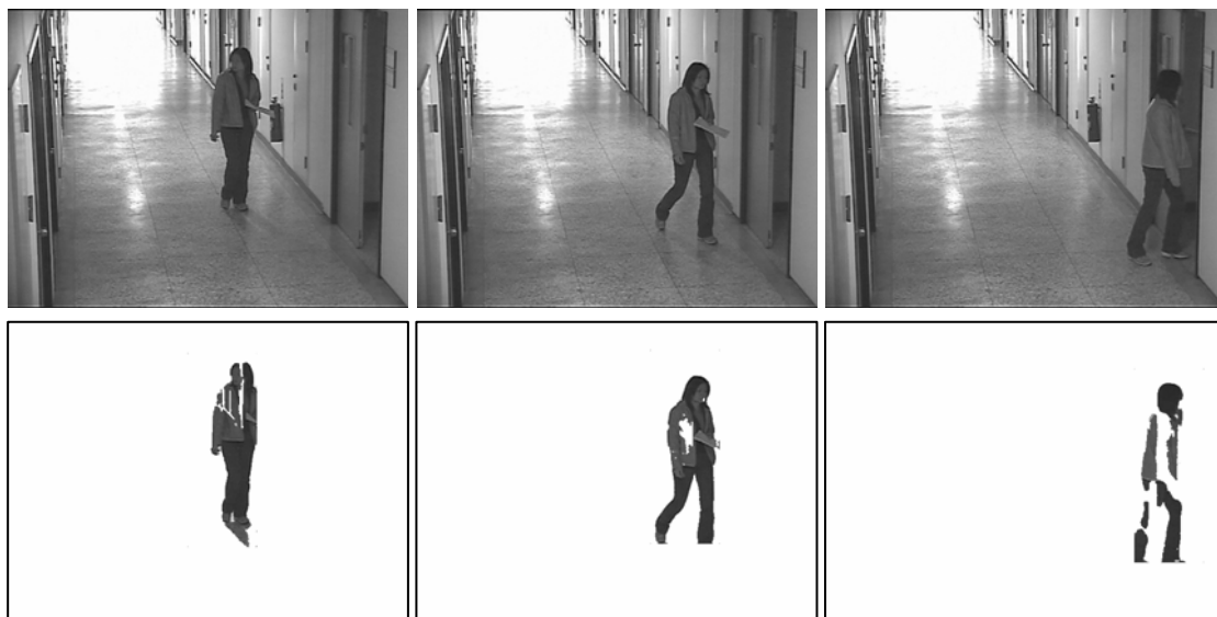
Fig. 2.1.1 (d1)(e1)(f1) Original images at (a) frame 23 (c) frame 26 (e) frame 29 (d2)(e2)(f2) Tracking results at (b) frame 23 (d) frame 26 (f) frame 29
