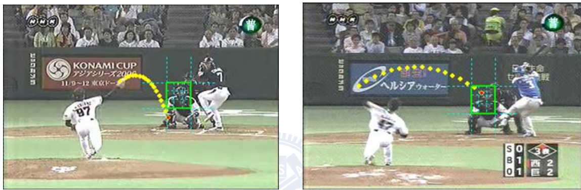
Fig. 4-8. Sample results of combining ball trajectory extraction with strike zone
