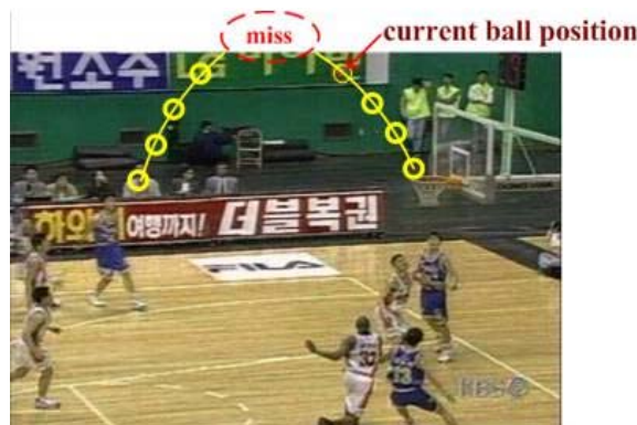
Fig. 2-19. Example of a shooting trajectory being separated.
