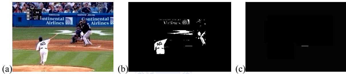
Fig. 4-12. Procedure of home plate detection: (a) Original frame of a pitch scene. (b) Pixels with high intensity around the frame center. (c) Detected home plate.
