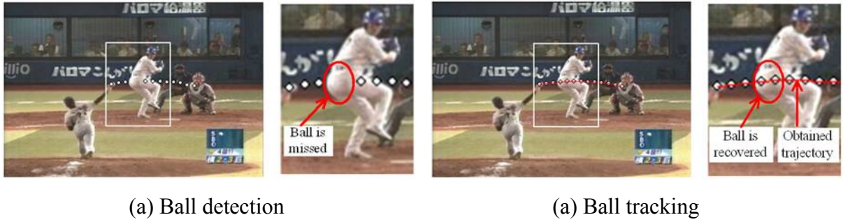
(a) Ball detection (a) Ball tracking Fig. 4-25. Illustration of ball detection and ball tracking in baseball video. (a) Ball detection. Two ball positions are missed when passing over the white uniform. (b) Ball tracking. Positions of missed balls can be recovered.
