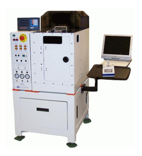
Fig. 4.8 Photograph of the Flip chip bonder.
