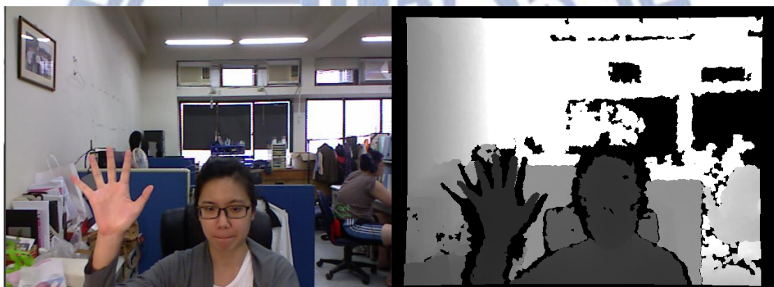
Fig. 4.2 The depth map with the non-overlap hand and face for ROI selection
