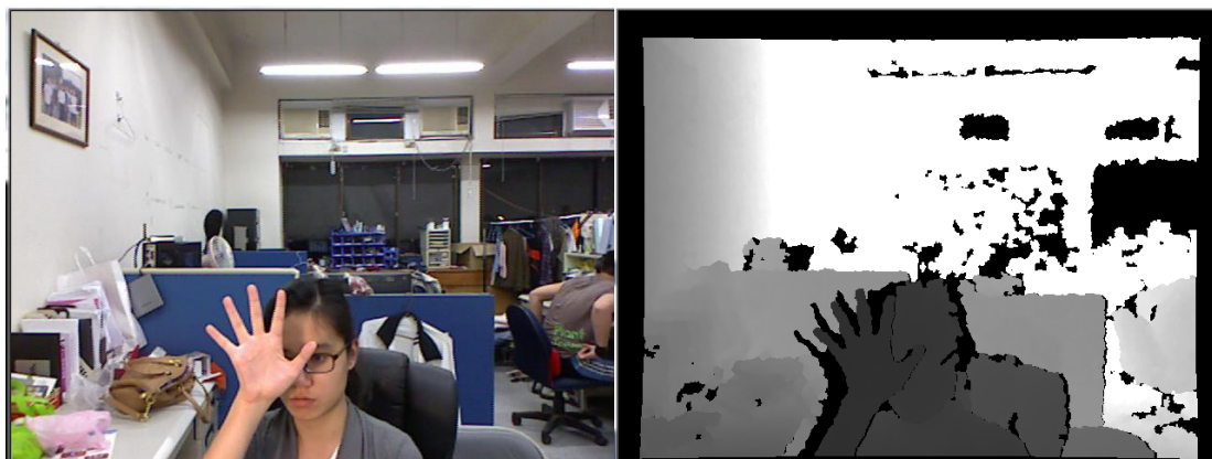
Fig. 4.4 The depth map with the overlap hand and face for ROI selection
