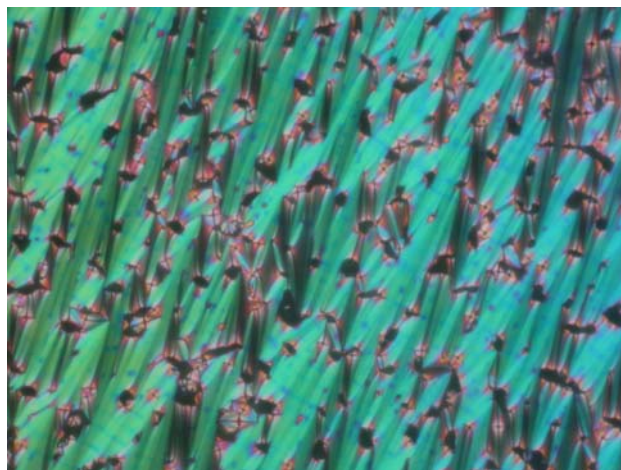
Figure 3.3 The optical texture of the mesophase ( S_A ) of P1 observed by POM at 270 °C (cooling).
