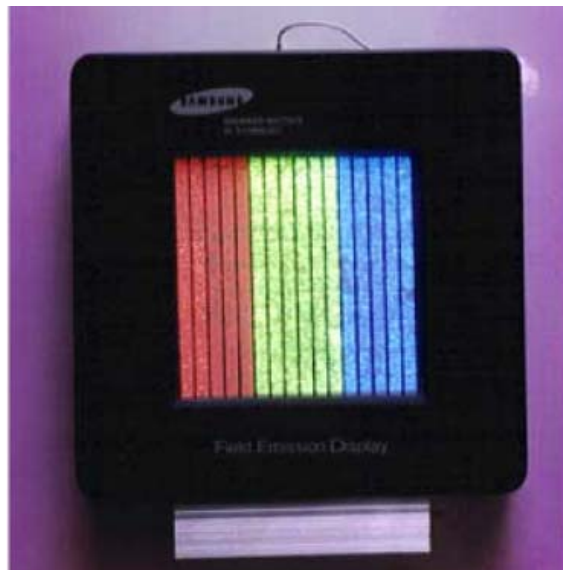
Fig. 2-6 A prototype 4.5 field emission display fabricated by Samsung using carbon nanotubes [Choi 1999-399].
