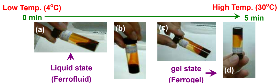
Fig. 7.3 Series image of thermo response behavior of ferrofluids: (a)&(b) liquid state (ferrofluids); (c)&(d) gel state (ferrogel)
