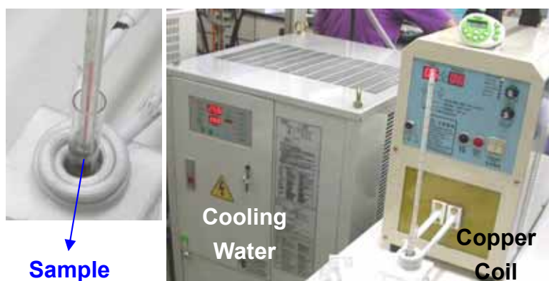
Fig. 3.1 Equipment of high frequency magnetic field
