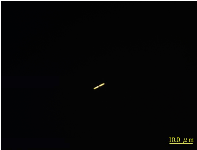
Figure10. The optical image of a Au-Ag-Au nanowire. Objective: 100× oil immersion lens.
