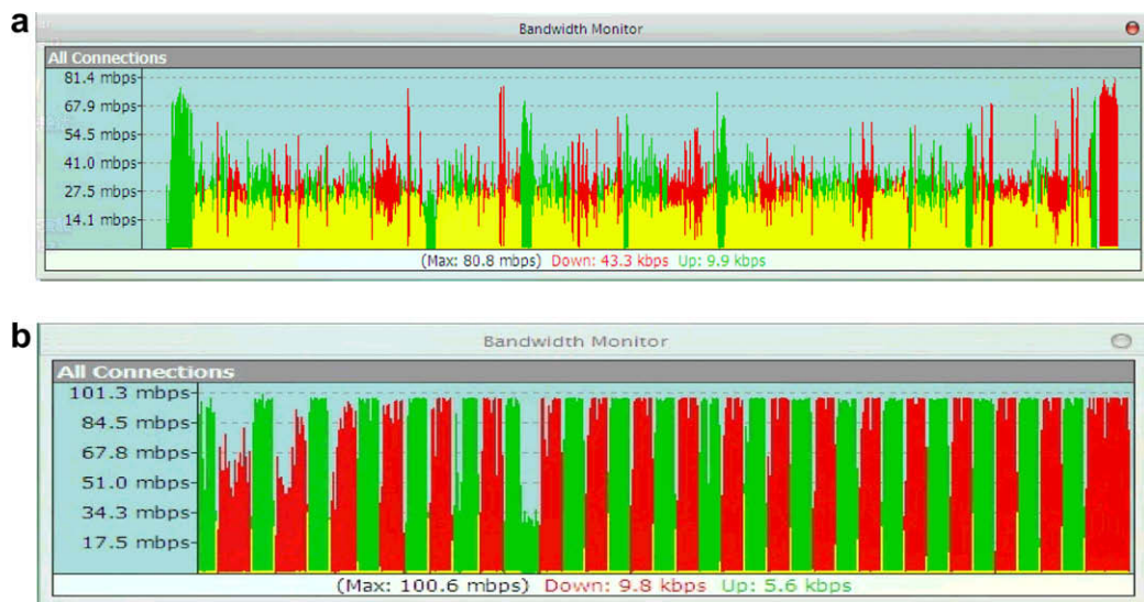
Fig. 23. (a) The network throughput demonstration without flow control mechanism. (b) The network throughput demonstration with flow control mechanism where red represents downloading flow, green represents uploading flow and yellow represents the flow of downloading and uploading at the same time. (For interpretation of the references in colour in this figure legend, the reader is referred to the web version of this article.)
