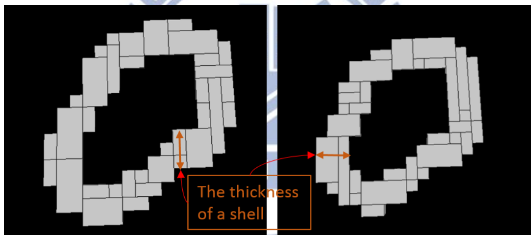
Figure 4.2: The structures of 7 th and 8 th layers of the bunny sculpture. The thickness is 3-unit-brick.
