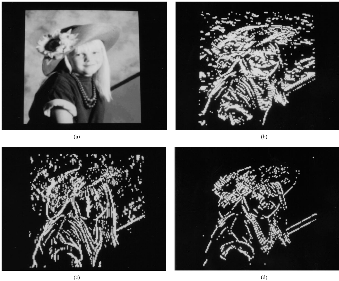
Fig. 6. (a) The lowest band x_{ll} . (b) The horizontal band x_{hl} . (c) The vertical band x_{lh} . (d) The diagonal band x_{hh} .
