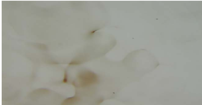
Fig 2-6-8 photoresist stripping by supercritical \text{CO}_2 with 9 % \text{PCO}_3 , 2 cycles of process step and 3 cycles of dry step
