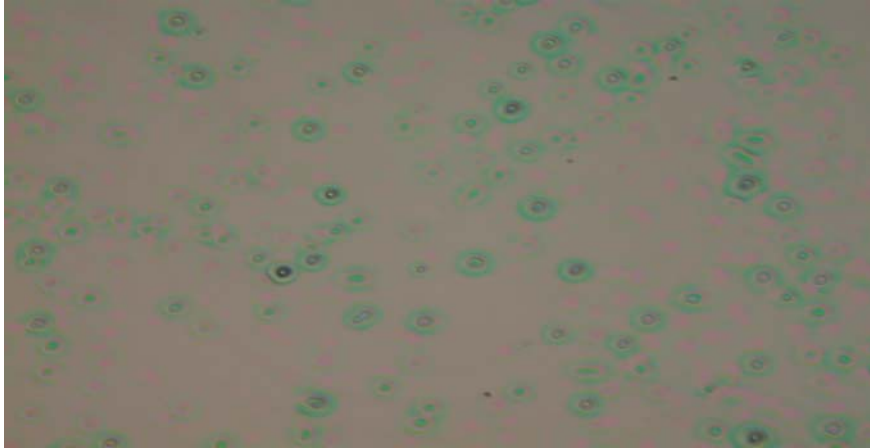
Fig 2-6-1 photoresist stripping by supercritical \text{CO}_2 with 1 % \text{PCO}_3 , 1 cycle of process step and 3 cycles of dry step
