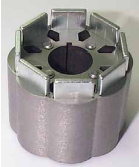
Fig. 2.3 Interior magnet type rotor L_d \neq L_q .
