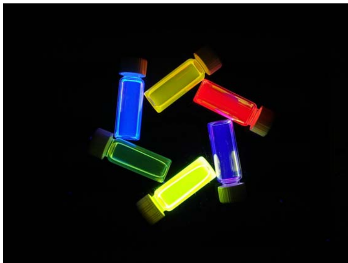
Figure 2.1: Emission color under UV illumination for colloidal CdSe/ZnS QDs with various sizes.
