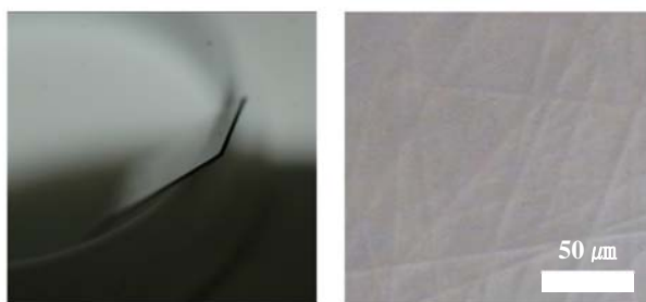
▼ The photo and OM image of N-face GaN after CMP process
