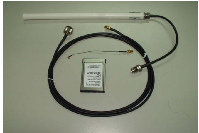
Fig. 19. The external antenna, cable, and wireless NICs used in the field trials.
