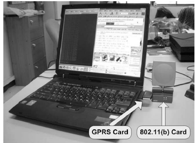
Fig. 10. Each notebook computer is equipped with an IEEE 802.11(b) WLAN interface card and a GPRS interface card.
