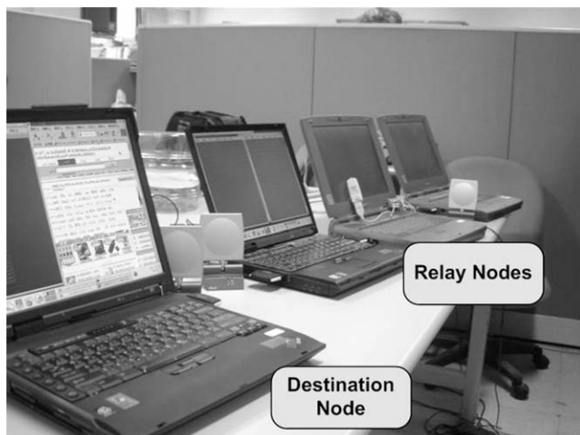
Fig. 9. Four notebook computers are used in experiments. One of them is used as the DN while the others are used as the DN’s helping RNs.
