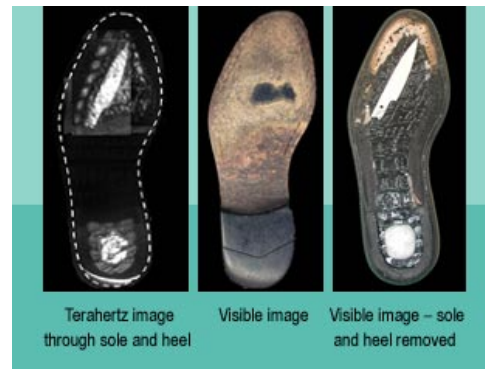
Figure 1.2: A demonstration of terahertz image through sole and heel.[1]
