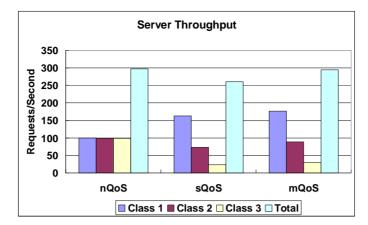
Figure 10. Server throughputs of the nQoS, sQoS, and mQoS scheduling.
