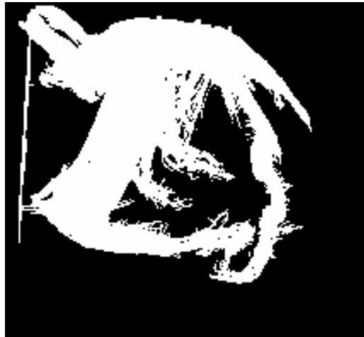
Fig. 5-9. The resultant binary image after the 2-D stencil masking process where the black pixel is denoted by zero and the white pixel is denoted by 1.
