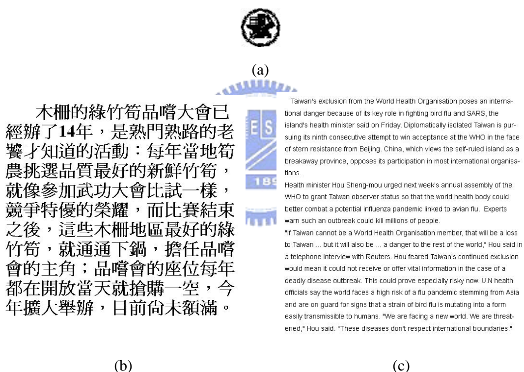
Figure 6.7 An embedded watermark image, input binary document images, output stego-images with authentication and watermark signals, and the differences. (a) A binary watermark image. (b) A binary Chinese document image. (c) A binary English document image. (d) and (e) Stego-images after embedding authentication and watermark signals. (f) and (g) The difference pixels before and after embedding authentication and watermark signals.
