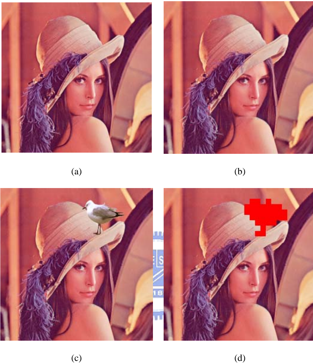
Figure 4.7 An example of results of applying proposed authentication method. (a) An image of “Lena”. (b) The stego-image after embedding authentication codes. (c) A tampered image of “Lena”. (d) Authentication result.
