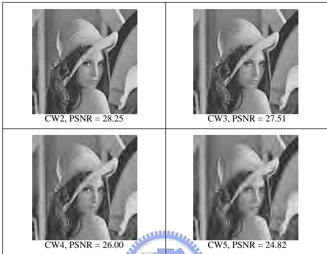
Fig. 4-8. Comparison of reconstructed Lena image using CW with different filter orders. ( D = 4 , CR = 30:1 )
