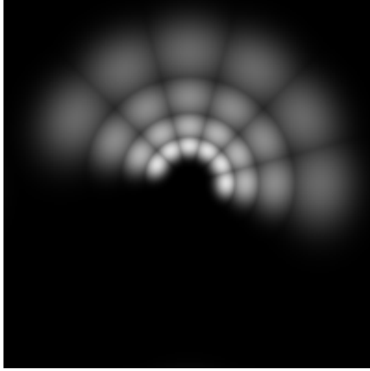
Fig. 3.5 Filter responses in the Gabor filter dictionary. The filter parameters used are U_h = 0.35 , U_l = 0.1 , K = 6 and S = 4 .
