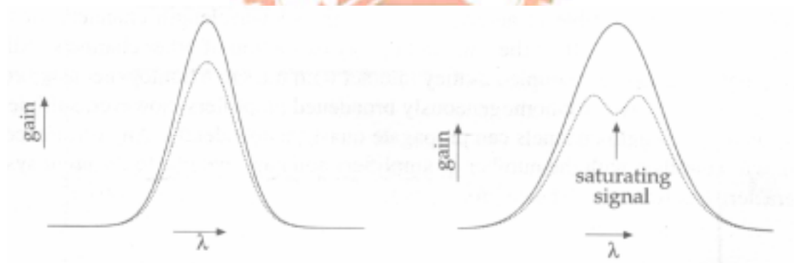
Fig. 2.3 Gain saturation for a broadened line (solid line: unsaturated gain; dotted line: saturated gain in the presence of a strong signal). Left: gain saturation for a homogeneously broadened line. Right: gain saturation for an inhomogeneously broadened line (the spectral position of the narrow band strong signal is indicated by the arrow).
