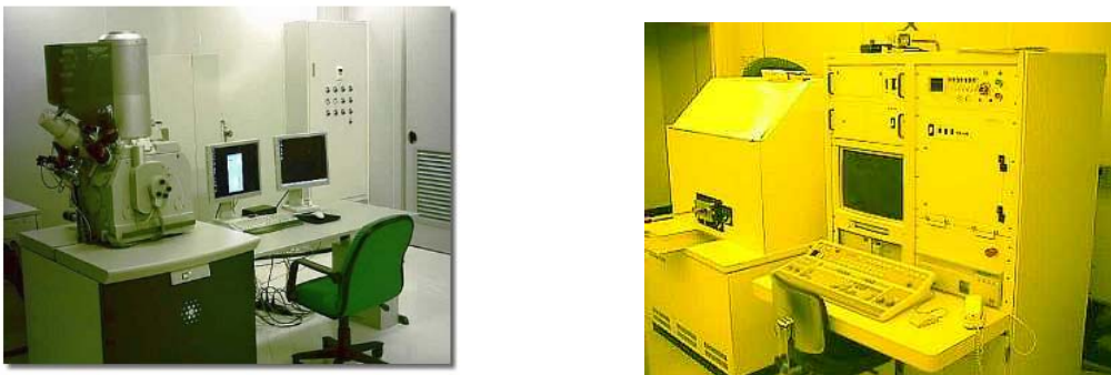
Fig. 5.1-2 Dual beam systems (FIB/SEM) in (a) PIDC and (b) CMU
