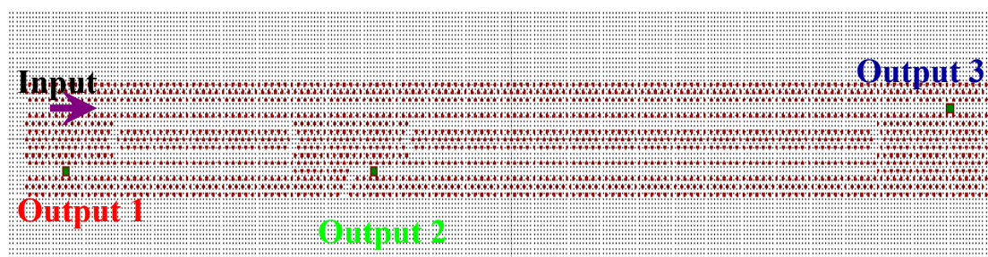
Fig. 3-19 WDM made up of two rings. There are two rings in the WDM. The coupling region of small one is 27 \Lambda . The coupling region of big one is 70 \Lambda .
