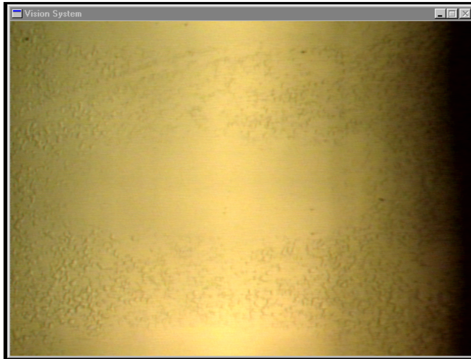
Fig. 3.9 (a) The surface of the etched thermally poled fused silica plate viewed under an optical microscope.
