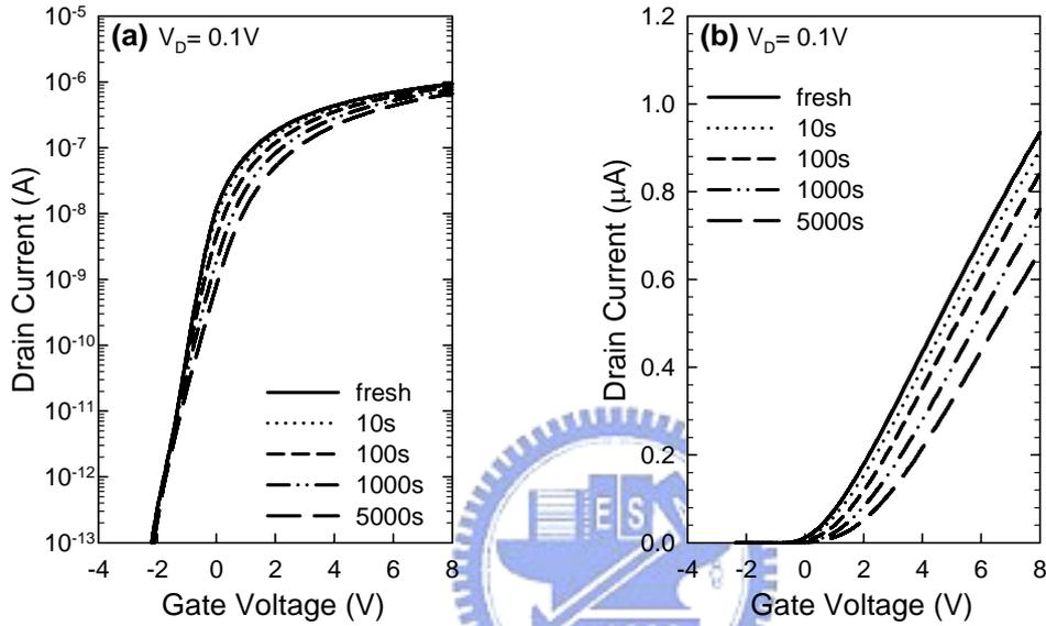
Fig. 6-11 Evolution of subthreshold characteristics of D-MT in (a) logarithmic and (b) linear scales during hot-carrier stressing under  $V_G/V_D=6.5V/13V$ .
