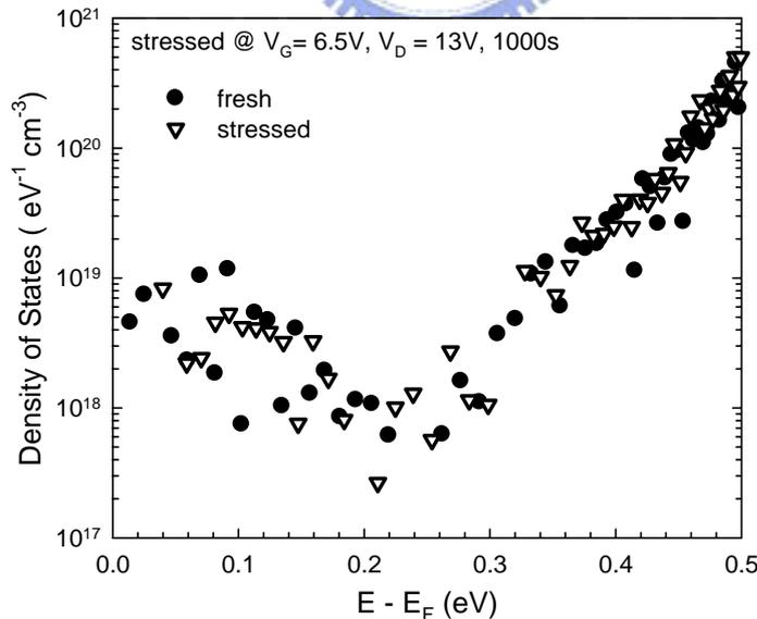
Fig. 6-7 Effective density-of-states distribution of TT before and after hot-carrier stressing under  $V_G/V_D = 6.5V/13V$  for 1000 sec.
