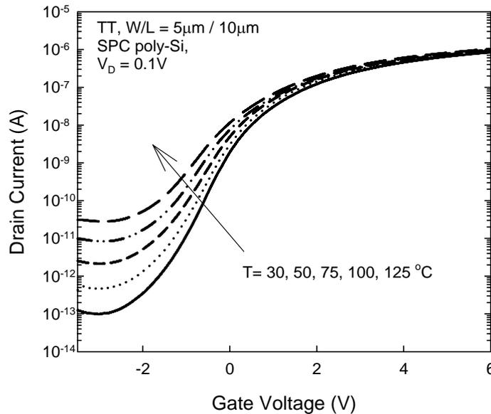
Fig. 6-1 Subthreshold characteristics of TT measured at different temperatures.
