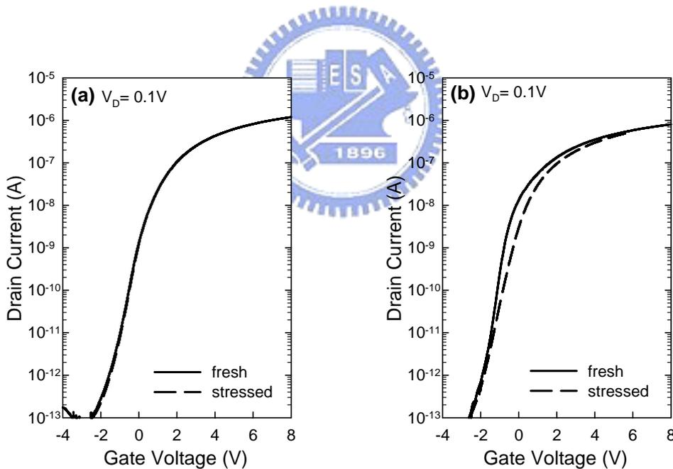
Fig. 6-6 Subthreshold characteristics of (a) TT and (b) D-MT, before and after hot-carrier stressing under  $V_G/V_D = 6.5V/13V$  for 1000 sec.
