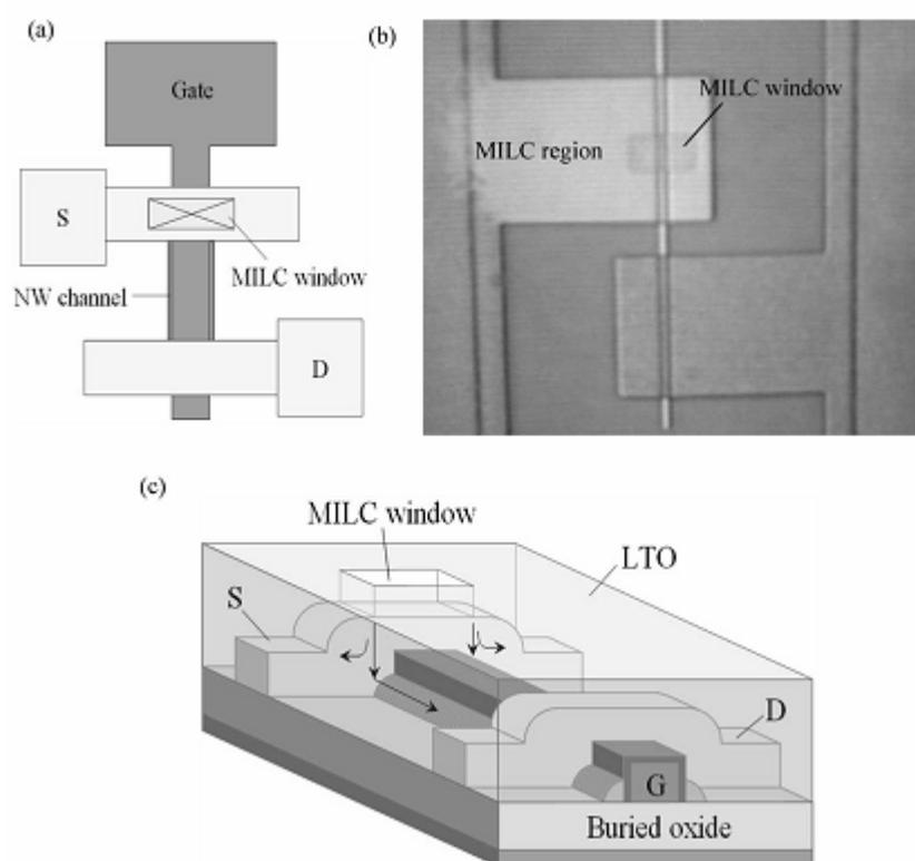
Fig. 7-1 (a) Top view of the layout, (b) the optical microscopy image and (c) the schematics of the poly-Si NWTFT enhanced by MILC.
