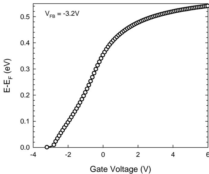
Fig. 6-3 Extracted surface band-bending as a function of gate voltage.
