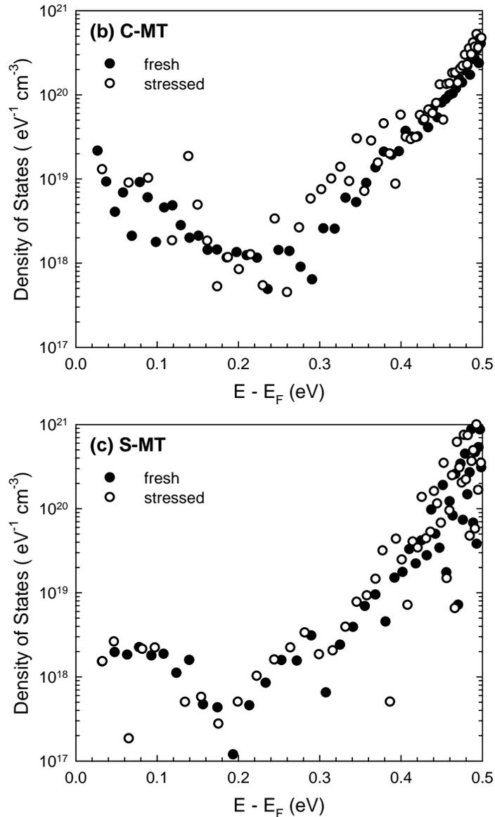
Fig. 6-15 Density-of-states distributions of (a) D-MT, (b) C-MT, and (c) S-MT before and after hot-carrier stressing at  $V_G/V_D$  of 10 V/20 V for 1000 sec.
