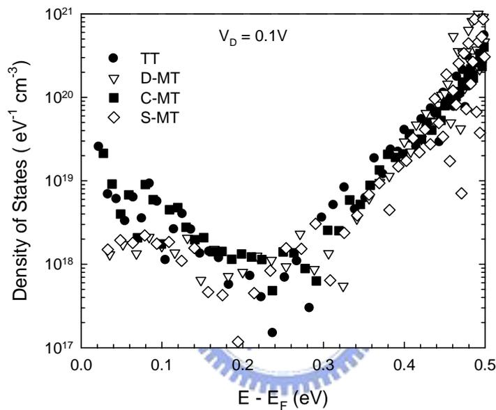
Fig. 6-14 Density-of-states distributions of the TT and three MTs before HC stressing.
