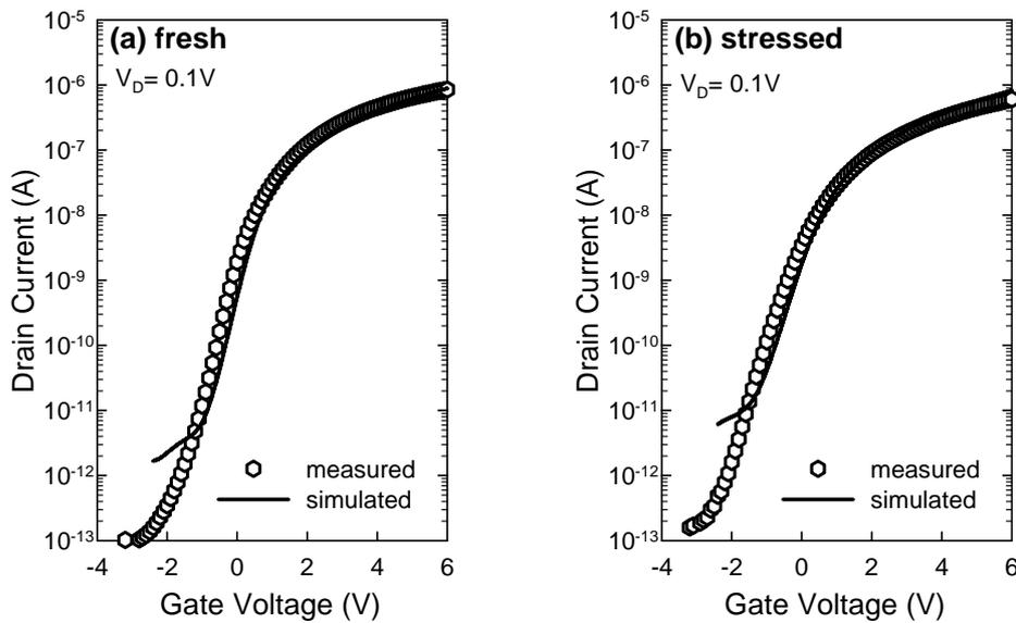
Fig. 6-17 Simulated subthreshold characteristics using data collected from MTs.
