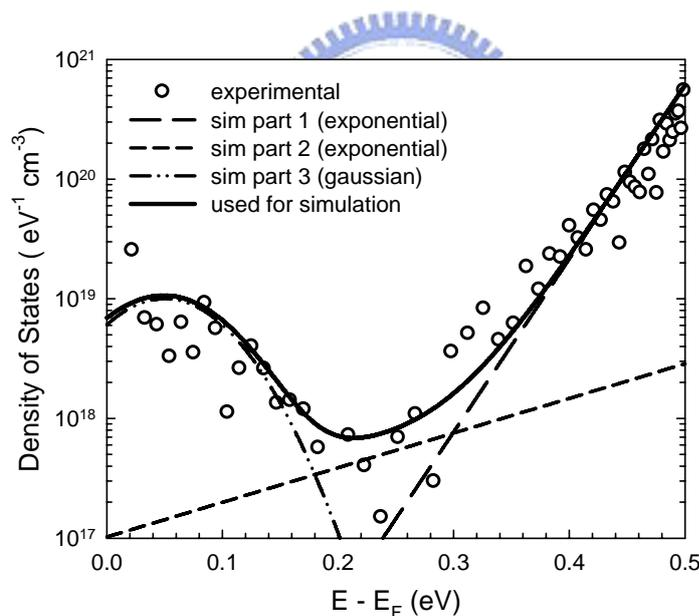
Fig. 6-5 One Gaussian and two exponential distributions used to represent the extracted DOS distribution.
