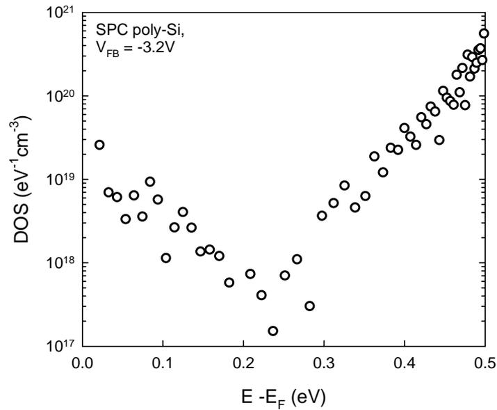
Fig. 6-4 Calculated density-of-states as a function of surface band-bending.
