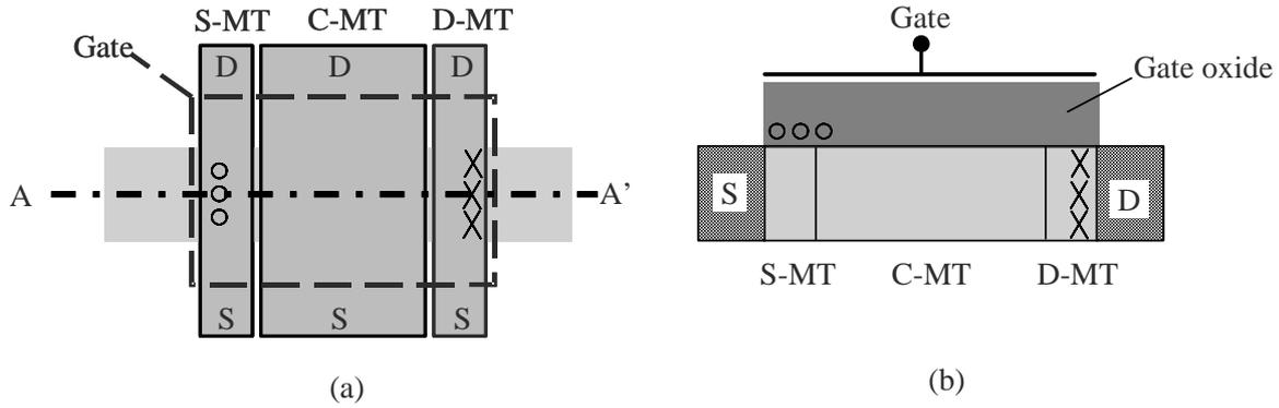
Fig. 6-16 Schematics of (a) top- and (b) cross-sectional view of the tester with indication of the induced damaged.
