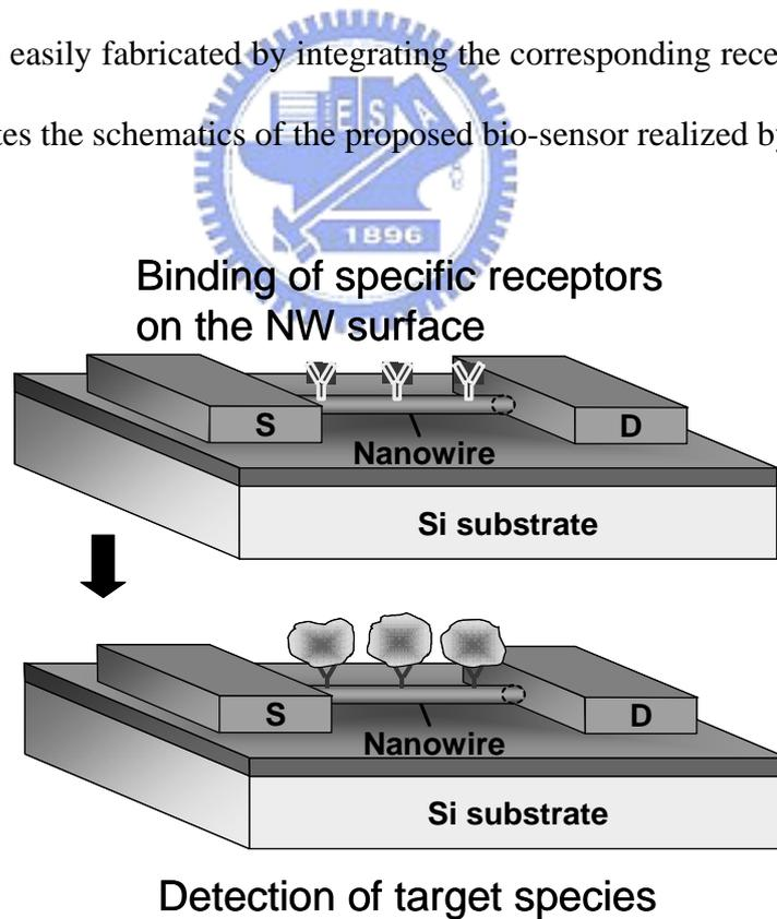
Fig. 7-2 Schematics of the proposed bio-sensor realized by the NWTFTs.
