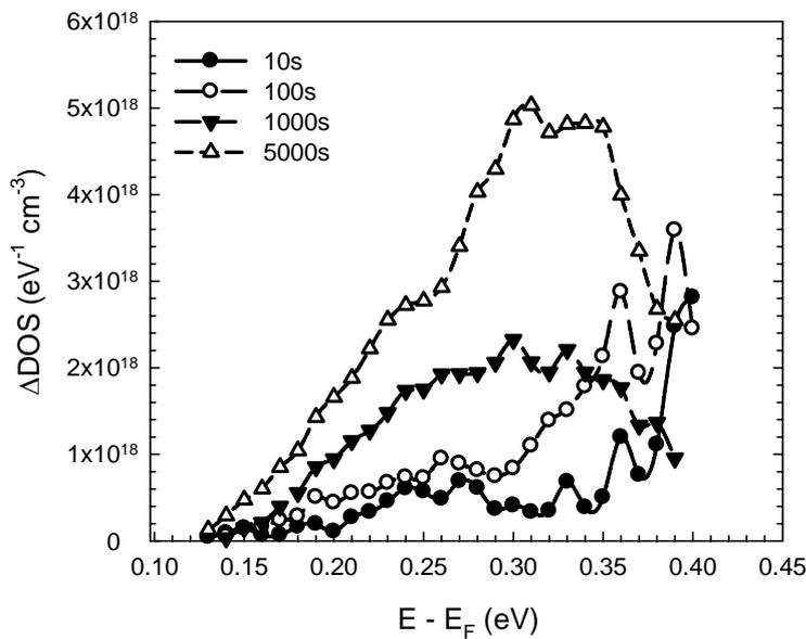
Fig. 6-12 Increase in density-of-states distributions of D-MT during hot-carrier stressing.
