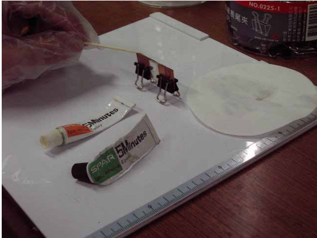
Fig. 3.11 Spread the AB glue all around in the sample
