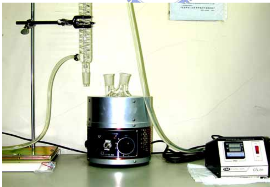
Figure 3.1. Experiment equipment used for fabricating ZnO quantum dots (QDS).
