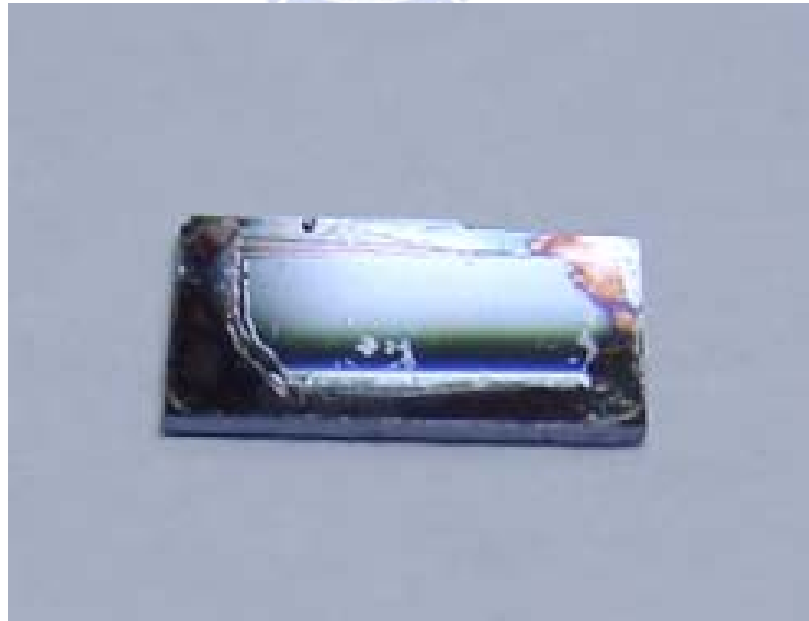
Figure3-3-4. A picture of the sample after glue bonding to DBR.
