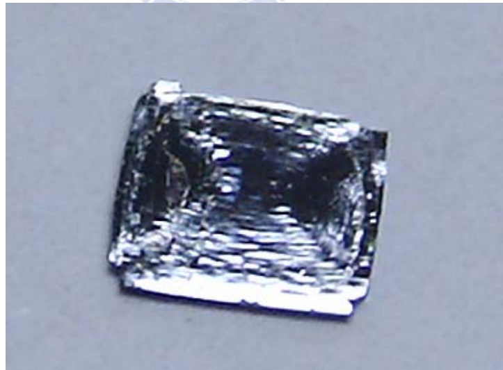
Figure3-5-5. The texture destroys the QW structure by diffusion.
