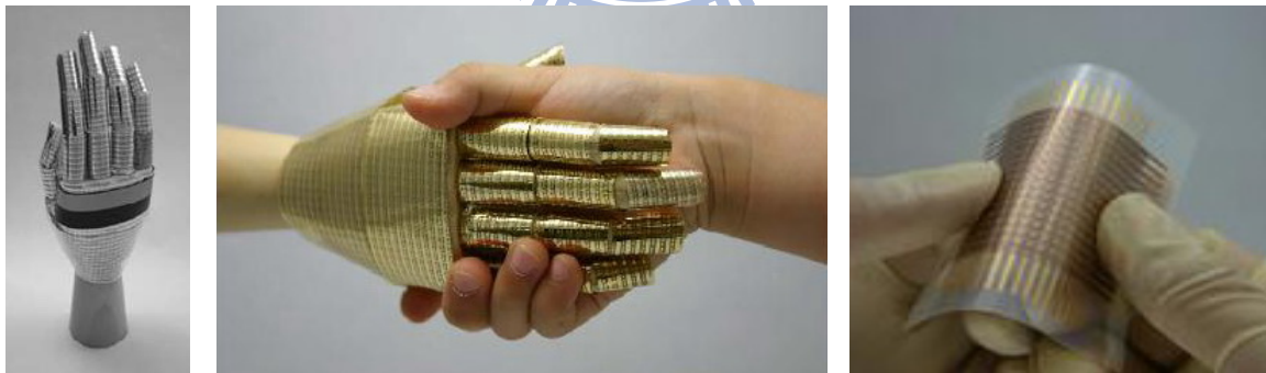
Figure 6-3. Electronics based on organic transistors of Takao Someya Group.
