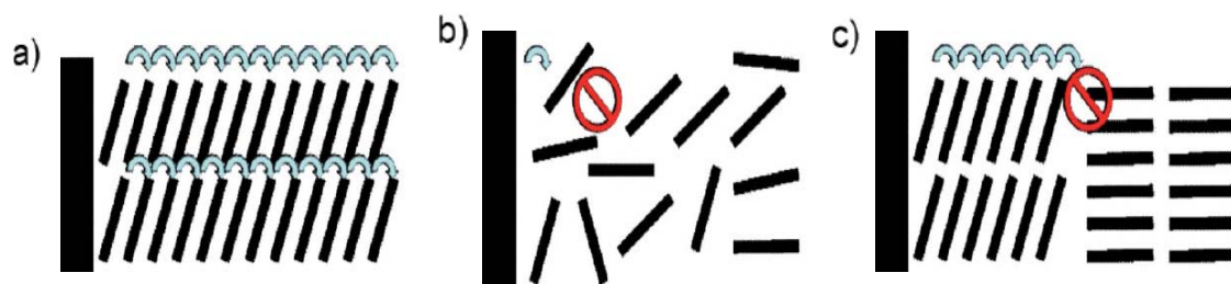
Figure 6-11. Charge transport in different orientations: a) crystalline-good charge transport; b) amorphous-no charge transport; and, c) polycrystalline-grain boundaries interrupt the charge transport.
