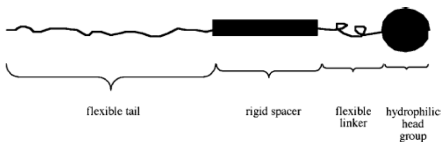
Figure 1-6. The divisions of an amphiphilic structure.
