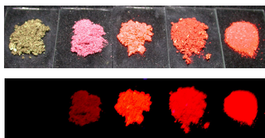
Figure 2-16. White light (top) and UV (bottom) illumination of the powder of Nile Red, DCM, pTFDCV , pTSPDCV , and PhSPDCV (from left to right), respectively.
