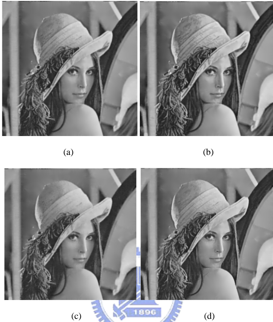
Fig. 5.20. Image contrast and sharpness altering. (a) Image with original contrast. (b) Image with enhanced contrast. (c) Image with softened contrast. (d) Edge enhancement.
