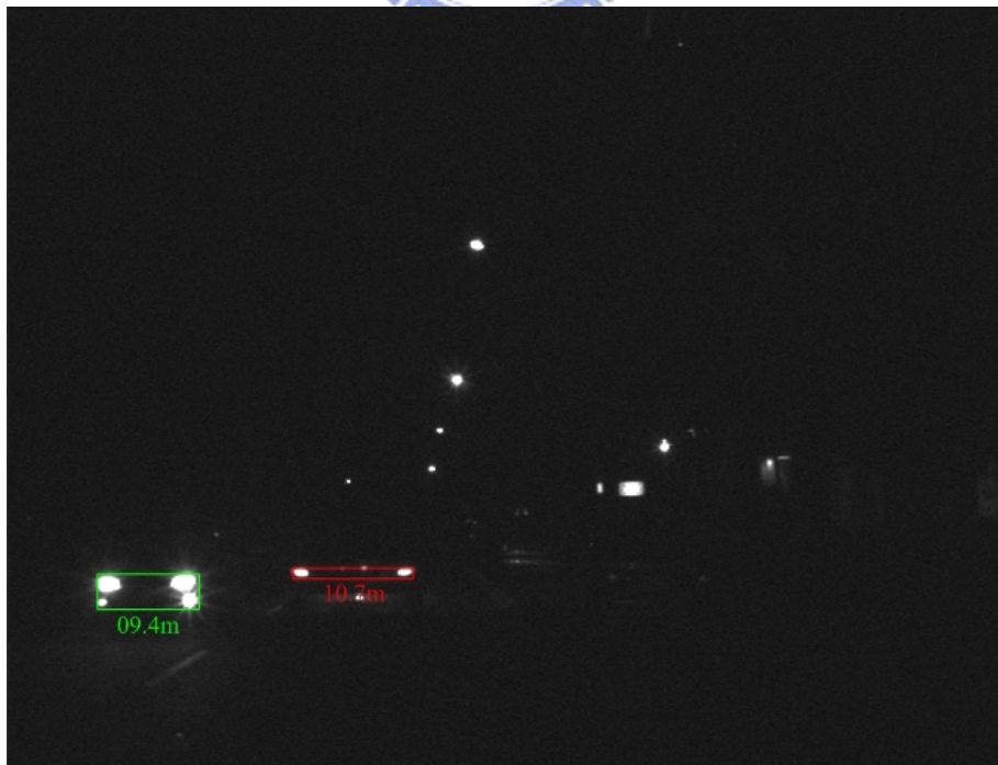
Figure 4.10. Result of vehicle detection on the nighttime road scene with both oncoming and preceding vehicles
