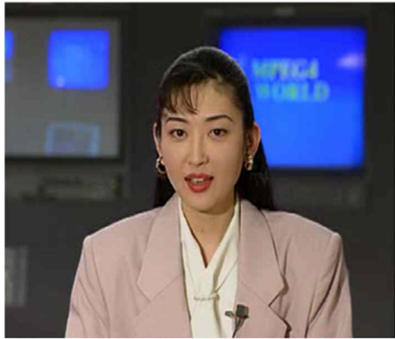
(b). Compressed image by MPEG-4 with compression ratio: 184
