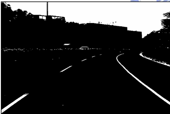
(d) The light object image derived by Between-class variance method
