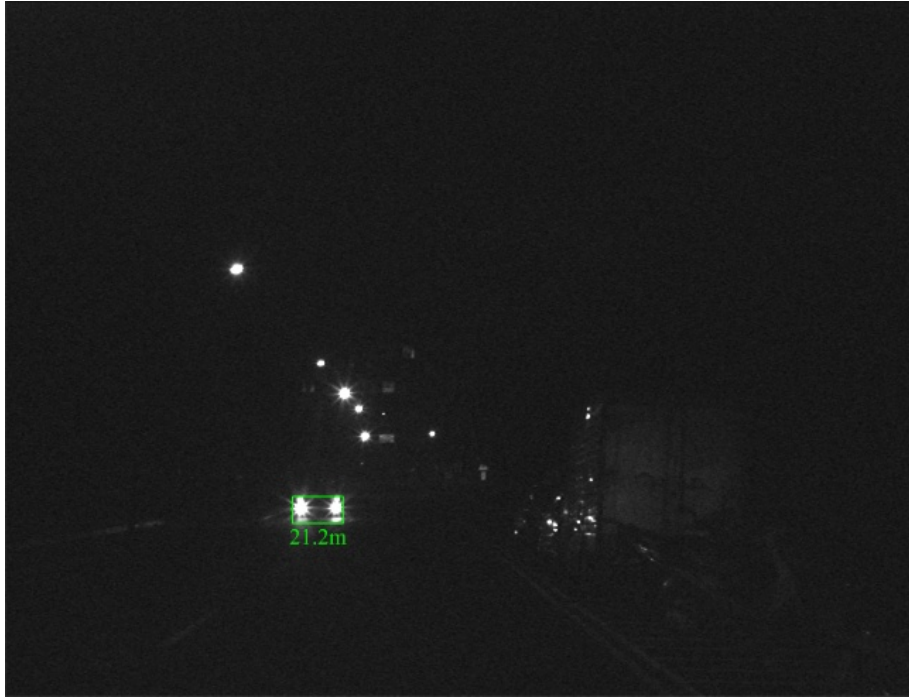
Figure 4.9. Result of vehicle detection on the nighttime road scene with one oncoming vehicle
