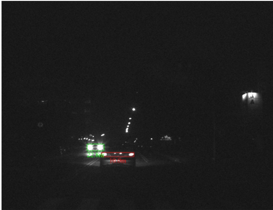
Figure 4.11. Result of vehicle detection on the nighttime road scene comprised of vehicles and many other non-vehicle lights
