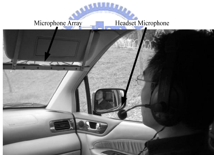
Figure 2-2 Installation of the array and headset microphone inside a vehicle
