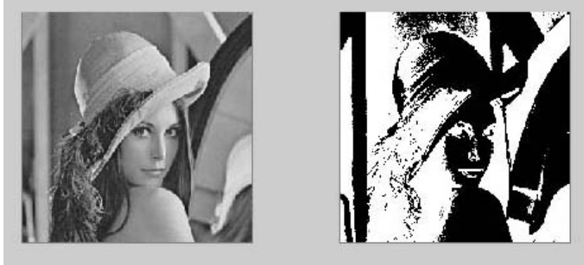
Fig. 2.2.3_1 Thresholding example by some specified template (Left: the original image, Right: the processed image)
