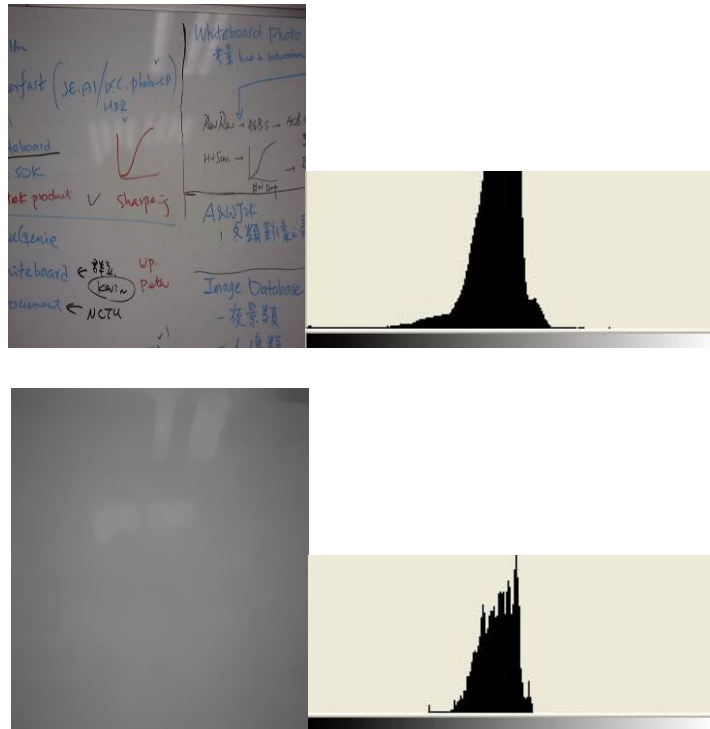
Figure 2.5 The first row shows original image and its histogram and the second row shows processed image by median filter and its histogram.
