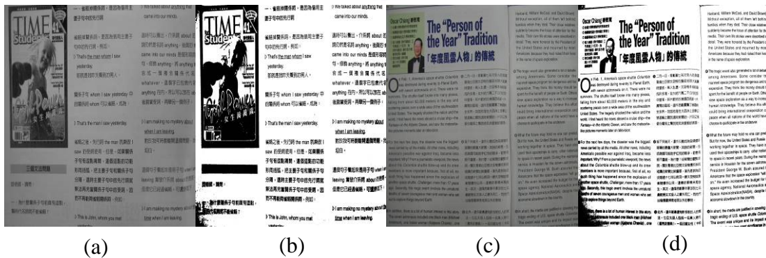
Figure 2.8 (a) and (c) are original images. (b) and (d) are processed images by global thresholding technique with Otsu's threshold selection algorithm.
