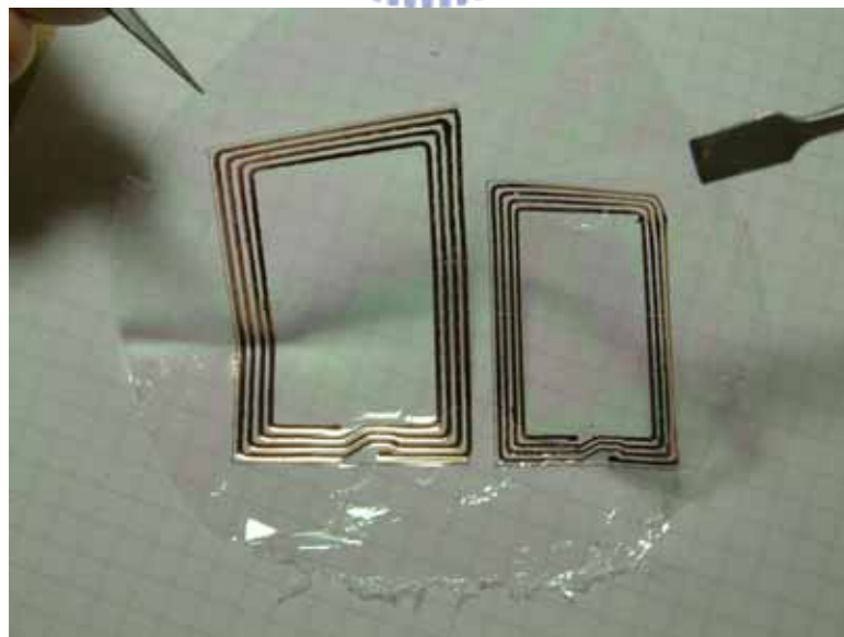
Figure 3-15: RFID antennas with different dimensions were fabricated on a flexible parylene membrane.
