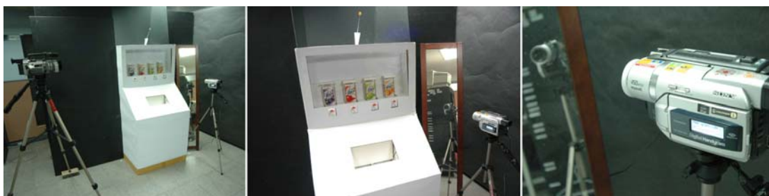
Figure 4.3 Experiment set up. The operation course was held in laboratory. Two cam-coders were set, one recorded whole behavior and process of task, another recorded subjects’ facial expression and connected with monitor behind prototype for operator.
