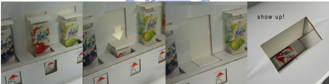
Figure 4.9 Getting Beverage Step a: Beverage moves down first and shows up in the outlet later.
