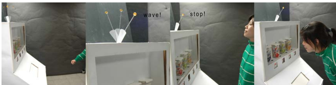
Figure 4.6 Approaching Step: Approach, stick wave, stick stop, subject choose beverages. When somebody approaches, the stick will wave. While being stared, it stops and waits for customers' choice.
