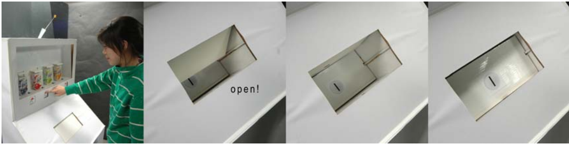
Figure 4.7 Ordering Step: Order beverages. Outlet's door opens. Slit plate lifted up. After customer chooses one beverage, the outlet's door will open and slit plate will then be lifted up to charge for order.
