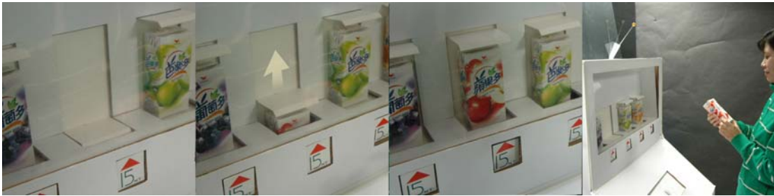
Figure 4.11 Leaving Step: New beverage moves up to the shelf. Stick wave. After customer take their beverage, new beverage move up to the shelf and then the stick wave to customers.
