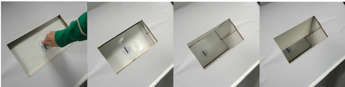
Figure 4.8 Paying Step: Pay for order. Slit plate move back. After receiving money, the slit plate then move back.
