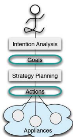
Fig 2-4: Principle of goal-based interaction (after Heider & Kirste, 2005).
