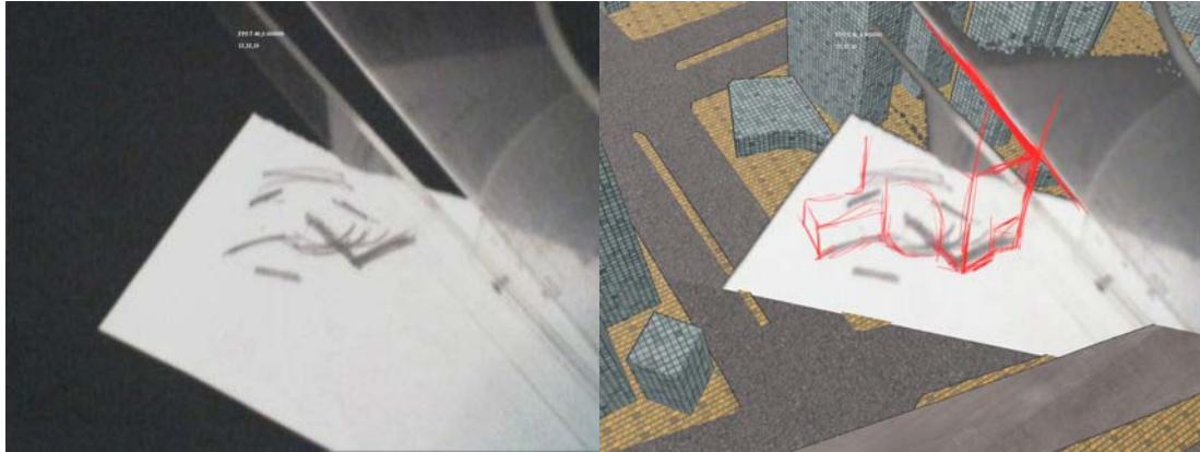
Figure 4.2.6: The image on the left is captured by the camera while designers using a right angle. Seeing the right angle while sketching can help designers easily sketch the correct perspective line (the image on the right).
