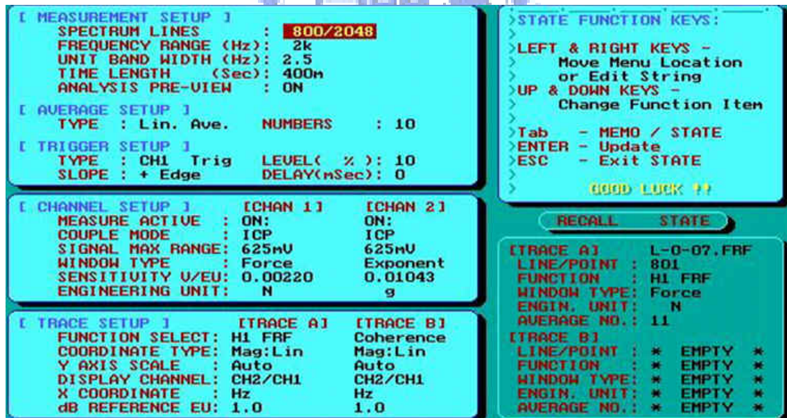
Figure 8. Parameters settings of hammer Impact testing
