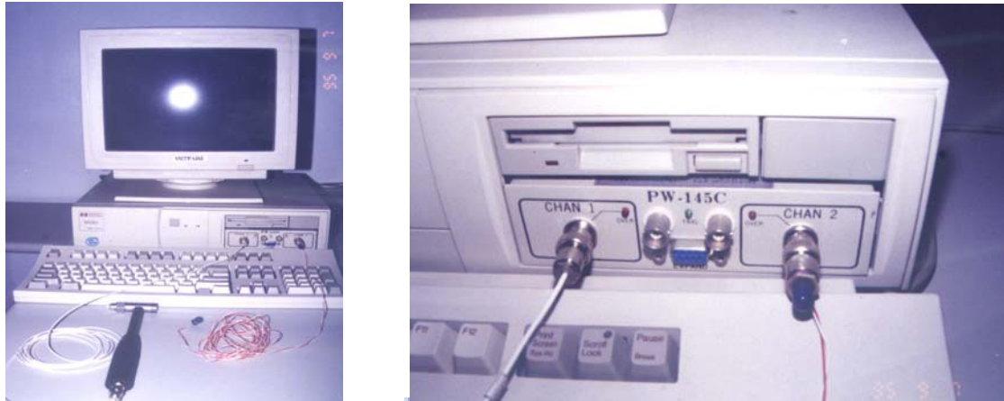
Figure 7. The PC base data acquisition system
