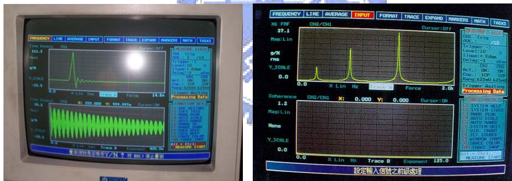
Figure 10. A typical test result for hammer impact test
