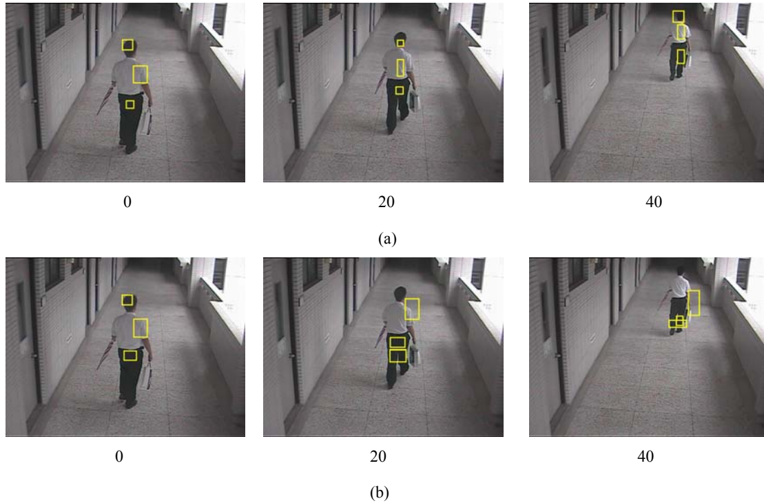
Fig. 6.14 The tracking results in a corridor. (a) Tracking results with failure detection and adjustment. (b) Tracking results without failure adjustment.
