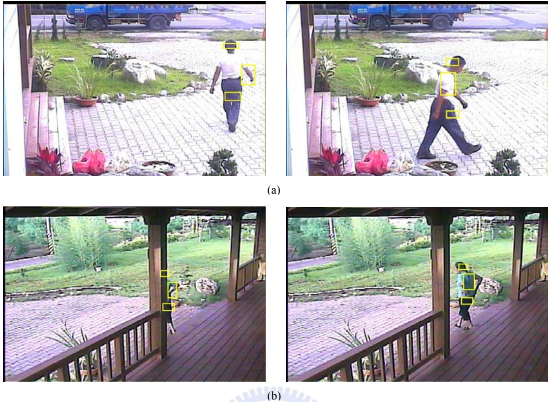
Fig. 5.3 Examples of two types of tracking failure. (a) A person with clothes colors similar to those of background regions. (b) A person occluded by a pillar.
