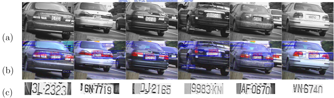
Figure 60: Examples of a variety of plates captured from a device installed in a car: (a) input images, (b) recognized results shown in color images, and (c) enlarged recognized plates.
