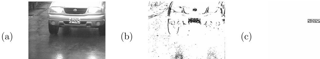
Figure 42: An example in which the one-pass plate extraction algorithm is applied: (a) Original image, (b) G_p of plate candidates, and (c) detected compact plate region.
