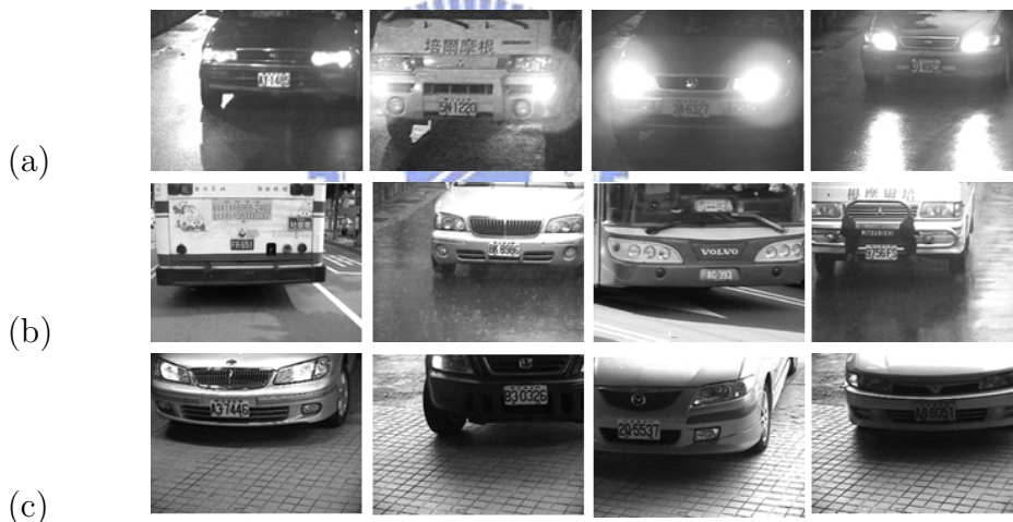
Figure 3: Examples of variations in plate types and environments: (a) different vehicle headlights, (b) different types of environment lighting, and (c) plate-like background.
