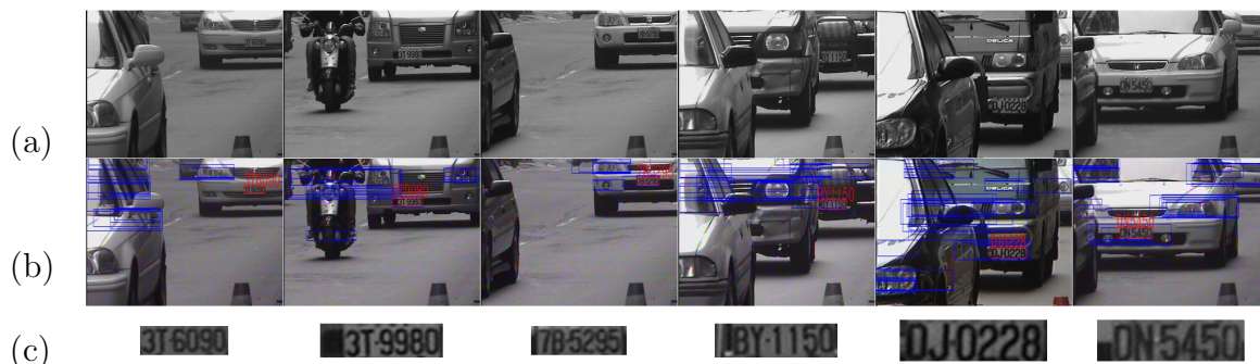
Figure 57: Examples of a variety of plates on a cloudy day: (a) input images, (b) recognized results shown in color images, and (c) enlarged recognized plates.
