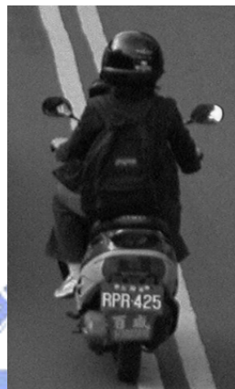
Figure 15: A license plate with unobvious borders. The plate and background have similar gray values.
