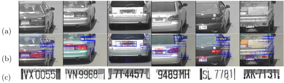
Figure 58: Examples of a variety of plates on a sunny day: (a) input images, (b) recognized results shown in color images, and (c) enlarged recognized plates.
