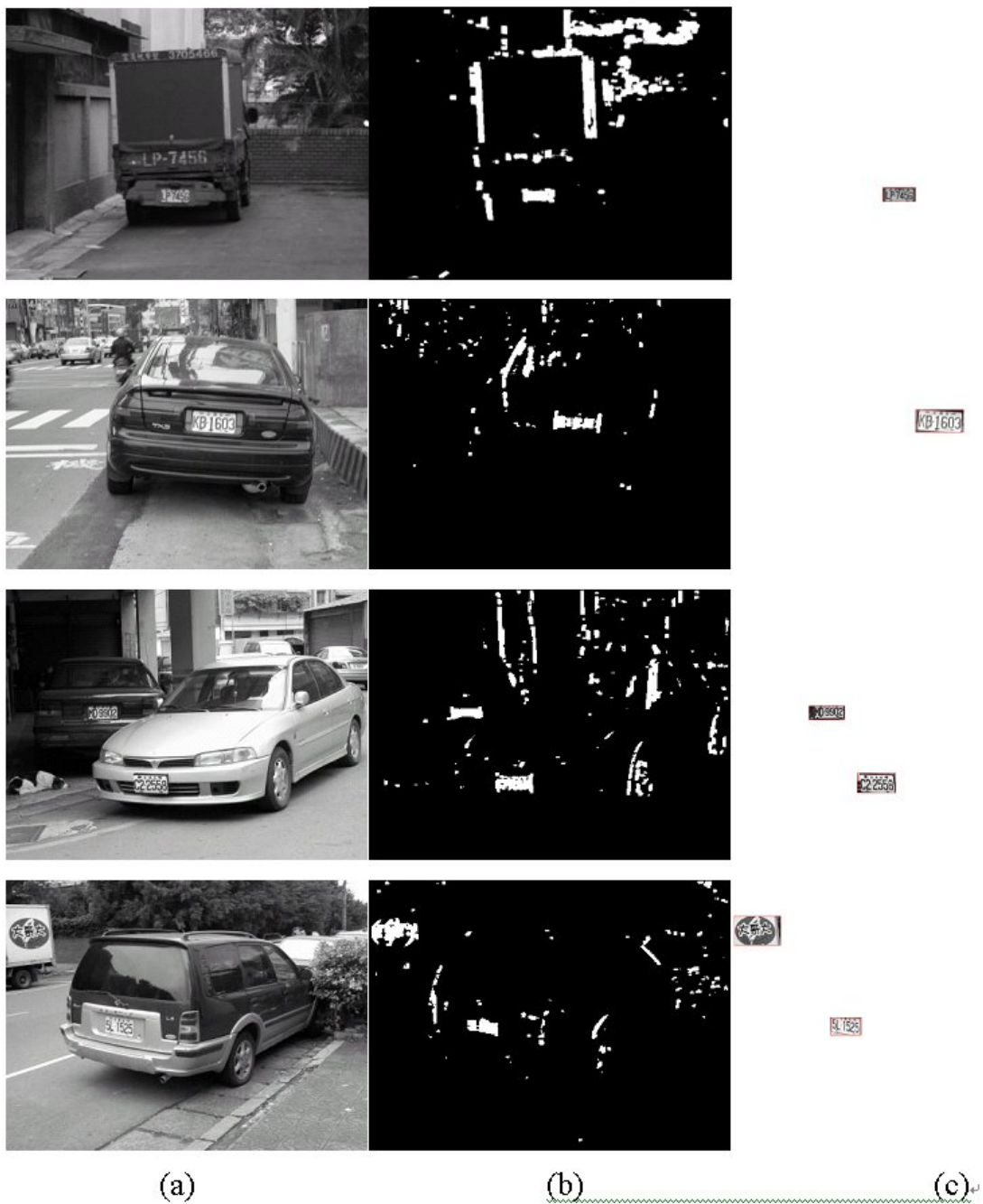
Figure 12: (a) The car images with license plates; (b) The possible license plate regions; (c) The license plate detection results.
