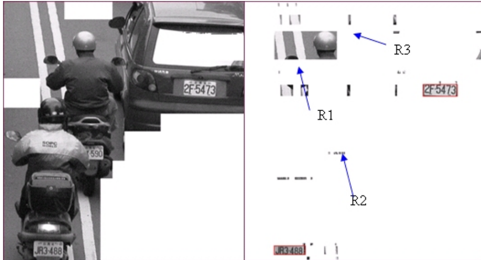
Figure 31: Candidate regions selection. Several regions are excluded since they do not satisfy the geometrical constraints.
