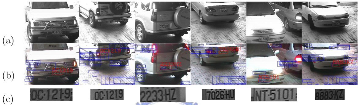
Figure 59: Examples of a variety of plates with the pavement background of texture patterns: (a) input images, (b) recognized results shown in color images, and (c) enlarged recognized plates.
