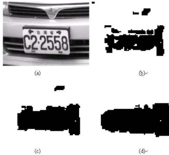
Figure 9: (a) The license plate image; (b)-(d) The possible license plate regions with the sizes of window mask, 7 \times 3 , 11 \times 7 and 15 \times 11 .
