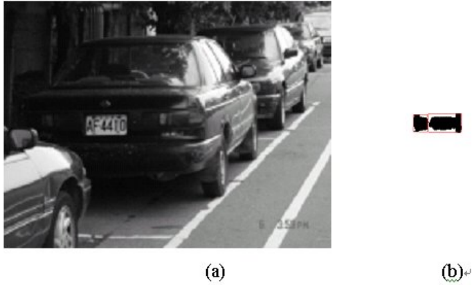
Figure 11: (a) The car image with a license plate; (b) The separated possible license plate regions.
