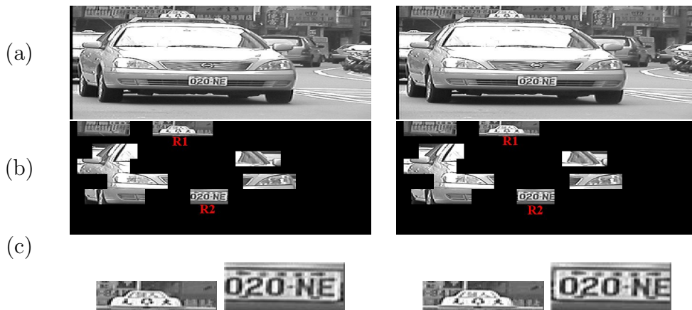
Figure 64: Examples of repeated regions in the same locations of two successive frames: (a) Left: the frame at time t - 1 , Right: the frame at time t , (b) the candidate regions in the two frames, (c) and the enlarged regions.
