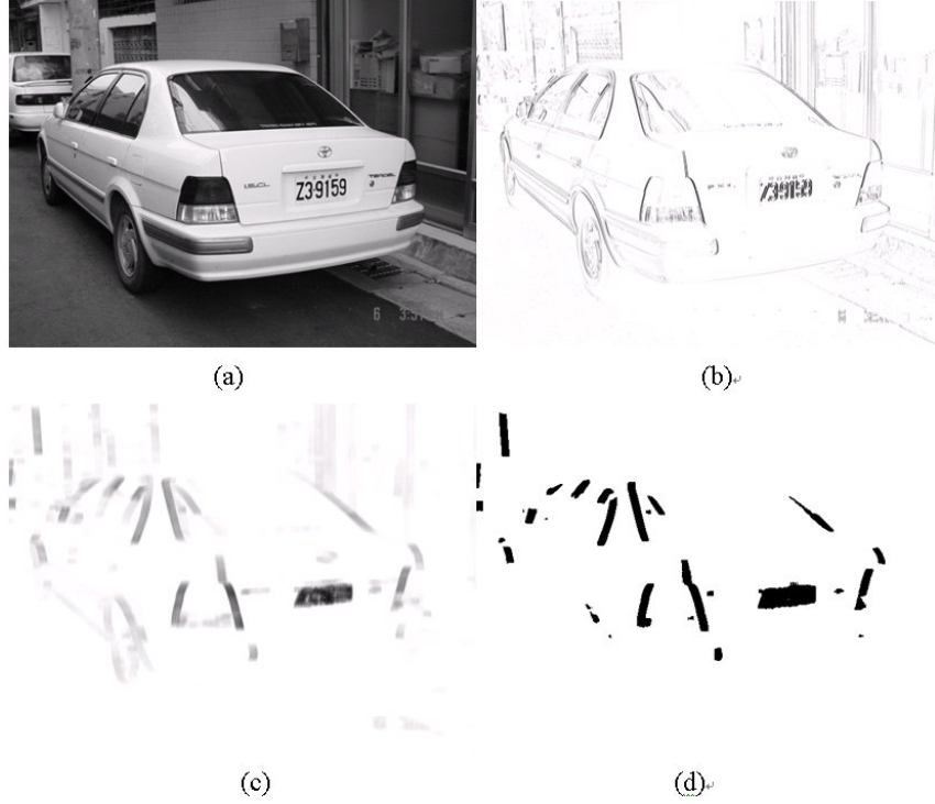
Figure 10: (a) The car image with a license plate; (b) The vertical gradients of Fig. 10(a); (c) The local variance of Fig. 10(b); (d) The possible license plate regions.
