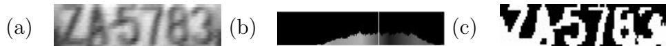
Figure 50: Inevident difference between the colors of the characters and the background: (a) compact plate region, (b) histogram, and (c) binary representation after thresholding by Otsu's method.
