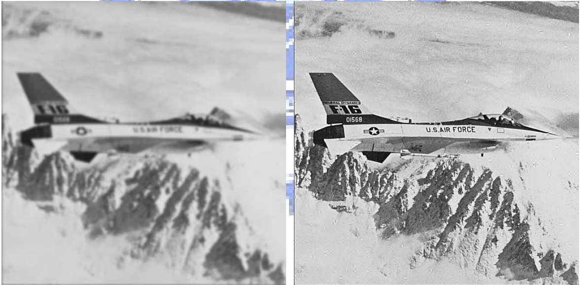
(c) Result image after Gaussian filtering. The PSNR comparing to watermarked F16 image is 26.6. The percentage of correct watermark bits is 68.84%. (d) Result image after sharpening. The PSNR comparing to watermarked F16 image is 25.42. The percentage of correct watermark bits is 99.21%.
