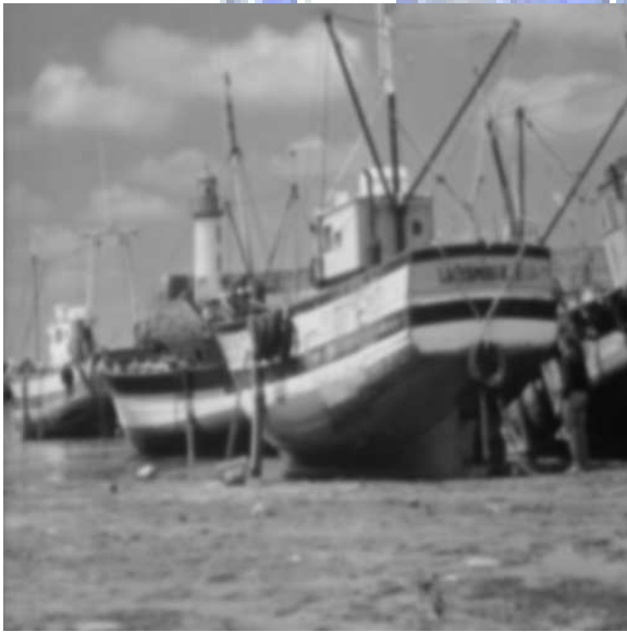
(c) Result image after Gaussian filtering. The PSNR comparing to watermarked Fishing Boat image is 25.59. The percentage of correct watermark bits is 66.99%.
