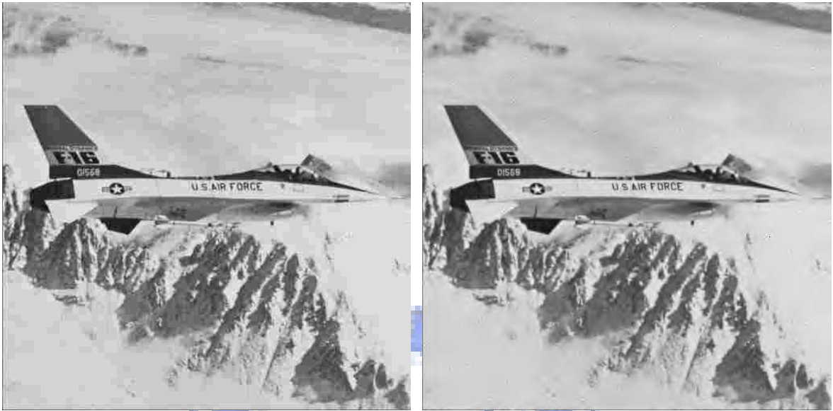
(a) Result image after JPEG compression. The PSNR comparing to watermarked F16 image is 30.39. The percentage of correct watermark bits is 60.25%. (b) Result image after JPEG2000 compression. The PSNR comparing to watermarked F16 image is 31.56. The percentage of correct watermark bits is 61.03%.
