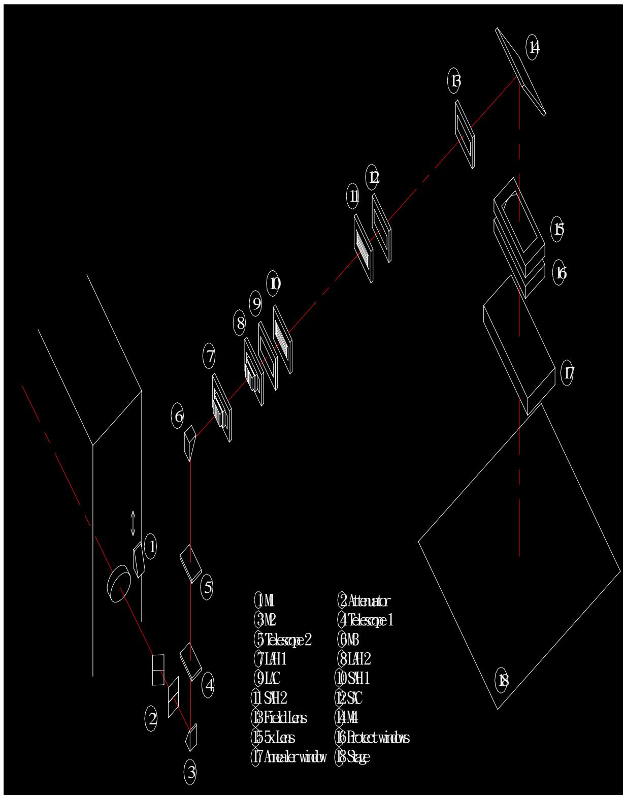
**Fig. 2-1** A brief schematic of the excimer laser optical system.
