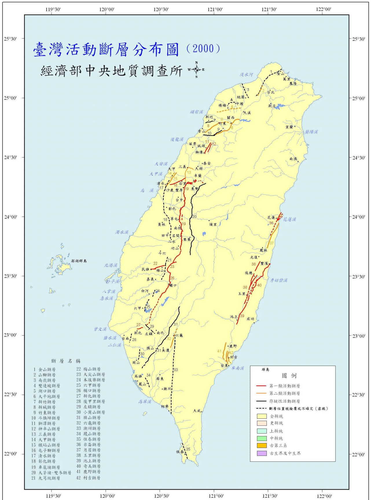
Figure 4-1 : Distribution of Taiwan Faults
